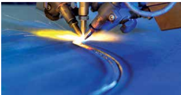
Oxy-Fuel Three Torch Contour Cutting
