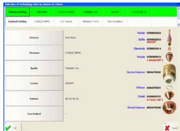
The Process Selector for the Process Database makes it easy to select material type, thickness, and quality, then the Vision T5 shows you which parts to put in the torch.
