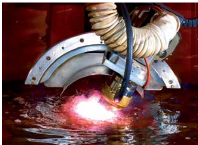
Plasma bevel cutting under water
