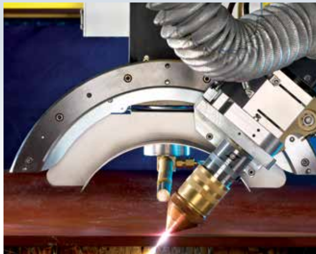
Plasma bevel cutting on a dry table
